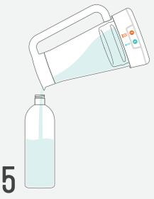
Unplug the Pro Appliance and pour your Force of Nature cleaner into the spray bottles. Rinse the Pro Appliance with water before plugging it back in. Press the start button twice in rapid succession to start your day counter.
