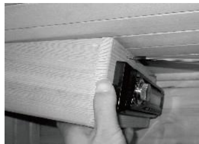
FIG 15.3 Screwing in the Radio Wood Housing
