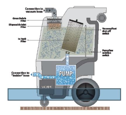
CAUTION! When cleaning, monitor foam in the machine's tank. Areas cleaned with other cleaning equipment or chemicals may cause excessive foam to collect in the tank.
