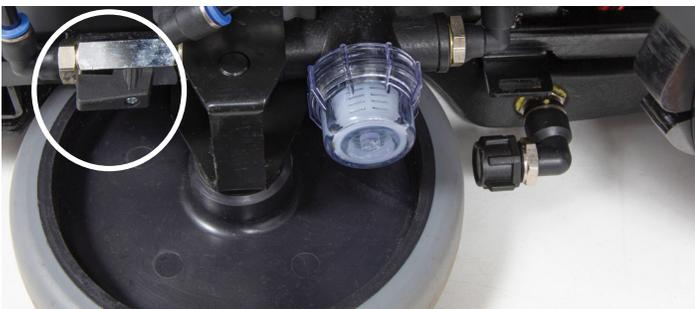
Fig 16 Solution tap fully closed
